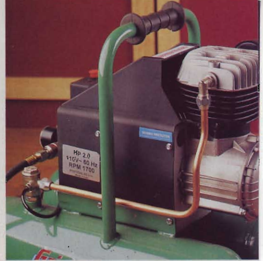
Unprotected copper tubing on the Grizzly could burn you if you pick up the compressor when it's hot. It's also more prone to dings and damage than Teflon tubing on other models.
